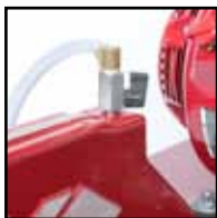
Adjustable water supply for wet cutting
