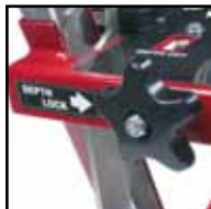
Positive-locking depth control mechanism
