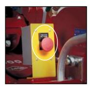
**Cutoff Switch** Gas engine cutoff switch is within operator reach from cutting position for quick shut down.
