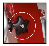
**Depth Lock** The cutting head can be locked in the down position when cutting smaller pieces and for consistent depth of cut.
