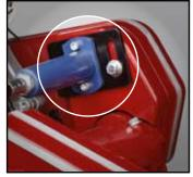
**Centrifugal Water Pump** Self-priming centrifugal water pump offers low maintenance. Easy to disengage for dry cutting.
