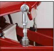
**Spherical Rod Ends**
