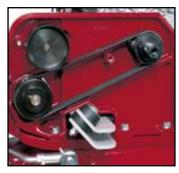
**Drive System** Micro V-Belt design drive system for more power transfer.
